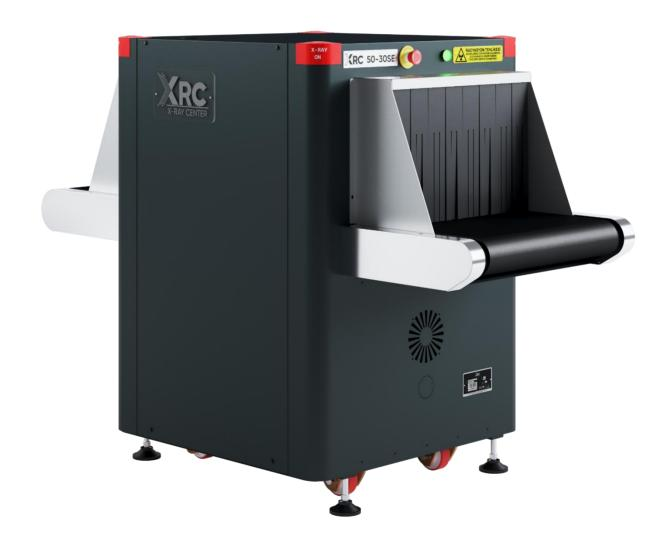
The XRC 50-30SE is one of the smallest tunnel sizes of the XRC baggage and parcel product range. It detects inorganic objects and provides an excellent image in an economical single energy (SE-Single Energy) diode array platform. It is a preferred model for locations with limited operating space.
